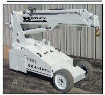
Fork Capacity: 2500 lbs. Hoist Capacity: 7200 lbs on main boom, 6000 lbs on telescoping boom. Panel Capacity: 1100 lbs Power: 24Volt 5HP Electric Motor. Controls: Walkie Handle or Radio Remote Control Boom: Base unit, 2 telescoping booms
