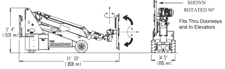
Three 180° Rotary Actuators Provide Precise Positioning
