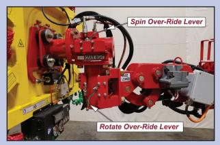
Manual over-ride for quick, precise adjustments
