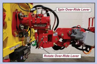
Manual over-ride for quick, precise adjustments
