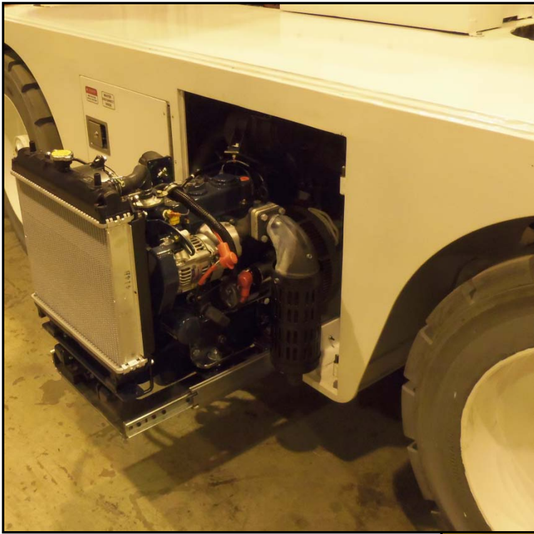
Hybrid Charging Engine on a pull-out engine tray for easy maintenance.
