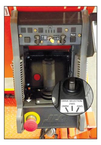
Unique Omni Drive Mode provides machine movement in all directions and for optimum positioning. Two wheel drive mode drives like an automobile for longer travel distances. Four wheel drive mode for tighter turning radius.
