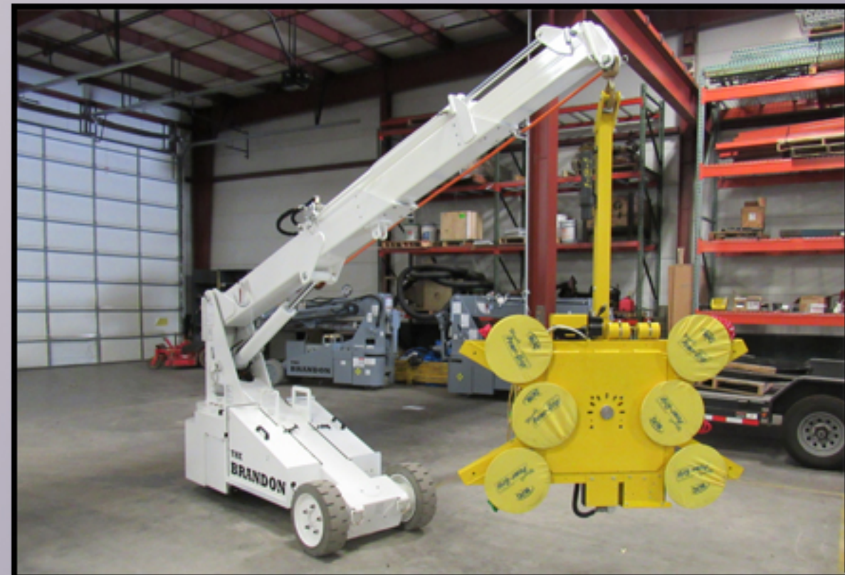
Glass Unit Pivot Bar Can be Installed for Hanging
